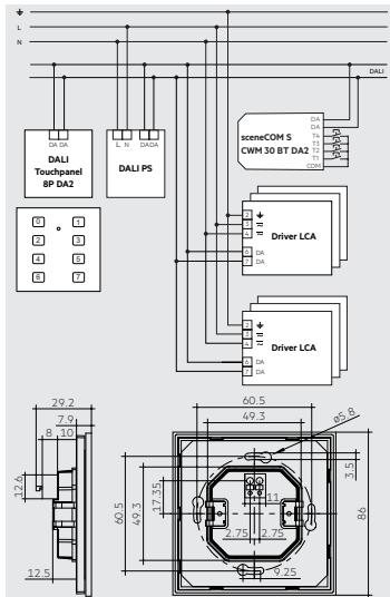
**UK** DALI-2 Bus powered Touchpanel with 8 push-button instances suitable for integration in DALI-2 Systems.
