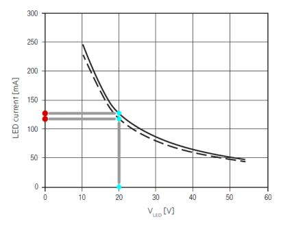
\_ The two crossing points are at around 120 mA (minimum value) and 130 mA (maximum value).
