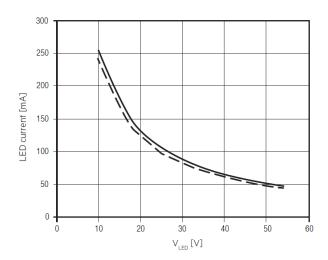
EM converterLED PRO 204 MH/LiFePO4 50V
