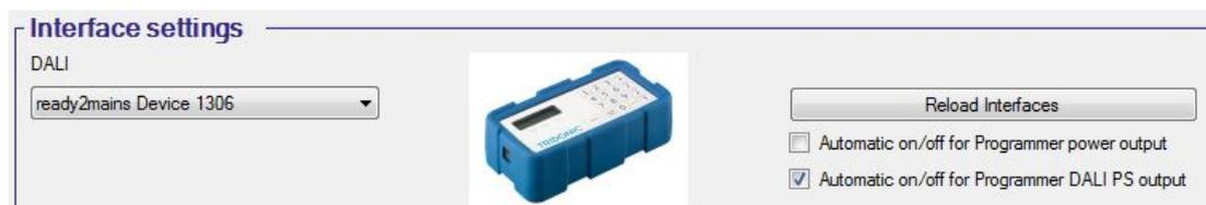
With the ready2mains Programmer it is possible to switch the power output and the DALI PS on or off.
