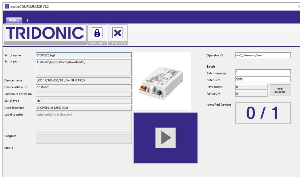
If the **Work** window is locked, it is also not possible to minimize or maximize the window. The buttons to do so are not available. It is necessary to set a password in the [Lock settings](#), p. 36!
