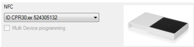
Activate the checkback **Multi Device programming** if more than one driver should be programmed at once.
