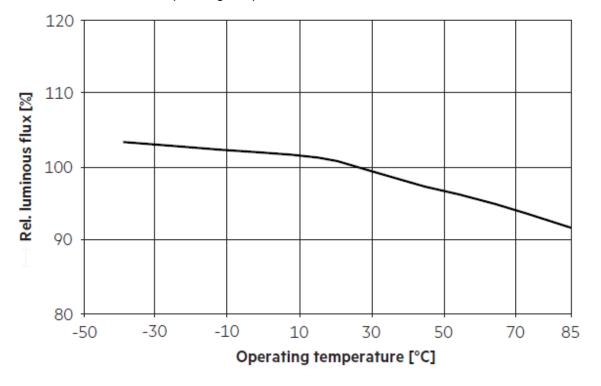
Relative luminous flux vs. operating temperature
