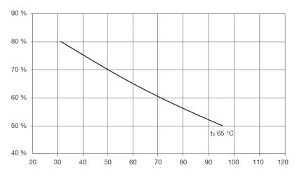
The diagram shows the change in luminous flux in percent over an operating time of 1,000 h at different tc operating temperatures.
