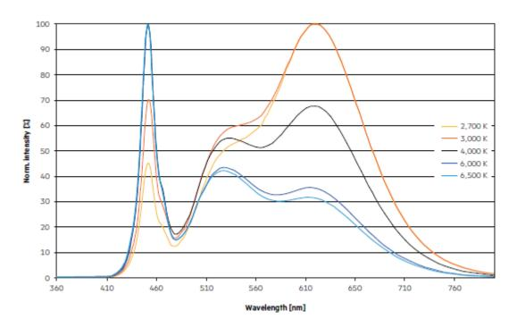
Colour spectrum at different colour temperatures
