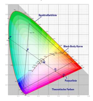
LEDs exhibit variations in terms of their exact shade of colour. This means that different "white" LEDs will all shine in a colour that is within the white colour spectrum. But the colours won't be exactly the same.
