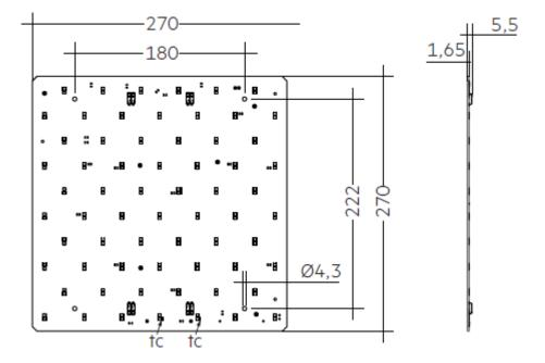
There is a t<sub>p</sub> point on top of the module for checking the temperature of the latter:
