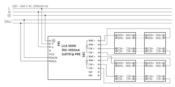
Wiring diagram switchDIM and colourSWITCH for QLE PRE (with 5 to 6 modules)
