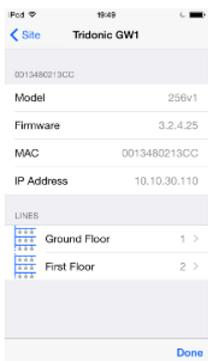
The LINES field is showing the connected DALI Lines. In this case there are two lines connected. Ground Floor which is connected to the first part of the connecDIM Gateway and First Floor which is connected to the second part of the connecDIM Gateway. One connecDIM Gateway supports up to four DALI Lines. The names Ground Floor and First Floor have been given already in the connecDIM Cloud, if no Cloud is used the Lines will just be named LINE1,2,3 or 4.
