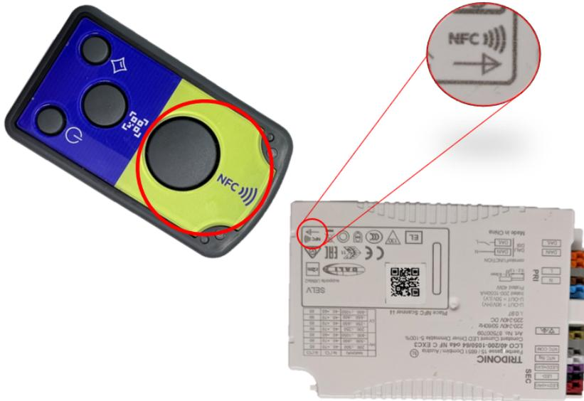
→ If the driver was programmed successfully, the green status LED will light up and the device will make a short beep sound.
